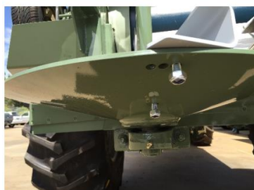
Short Vane on LH Spinner
