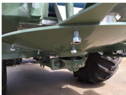
Long Vane on LH Spinner
