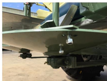
Short Vane on RH Spinner
