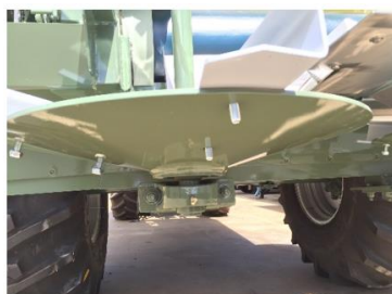
Long Vane on LH Spinner
