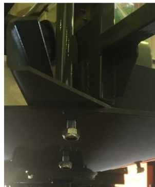
Long Vane on RH Spinner
