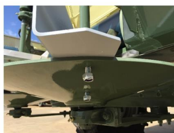
Long Vane on RH Spinner
